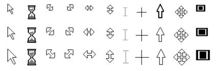
**System cursor colors.** This chart shows the effect of a color change on the system cursors (also known as mousepointers). You can change cursor colors by choosing from the cursor color pad in the Desktop ToolPanel. Note: Not all display cards support cursor color switching. If yours does not support this feature, the color pad won't appear in the ToolPanel.
